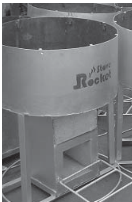
Figure 7 WFP type of stove: lower skirt, less L-shape at the entrance to cut costs, designed for half-220l gallon oil drum (photo: Christa Roth)
